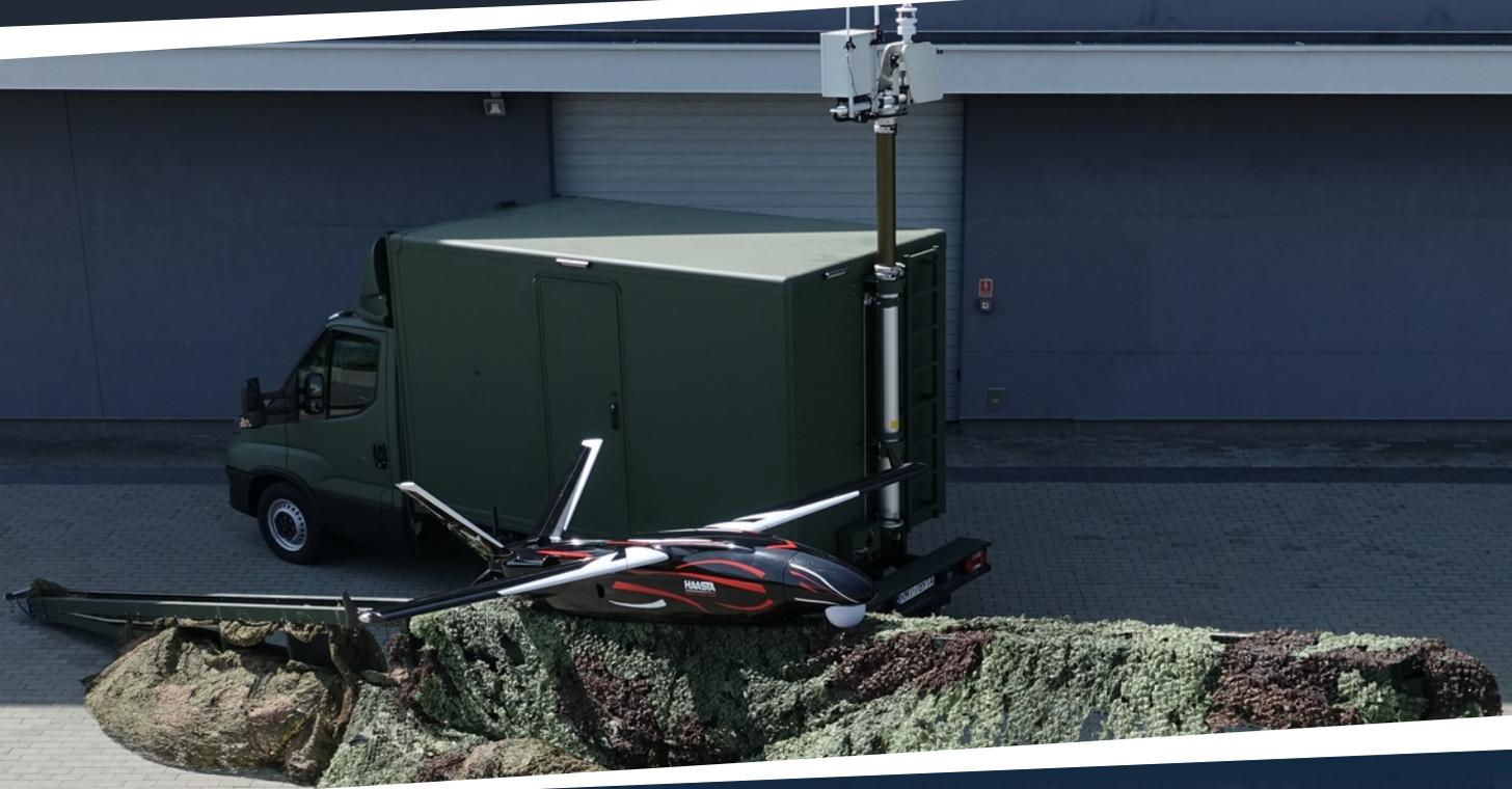
The HAASTA Aerial Target System is developed to provide a complete system capable of simulating different aerial threat and realizing various scenarios for effective training.
